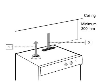
Ventilation out into the room where the drying cabinet is located. Drying cabinet not built in
